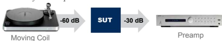
*When using a Hafler SUT with a preamp without a phono input, connect the SUT to a Hafler PH60 phono stage to introduce the RIAA equalization curve and extra gain.*
